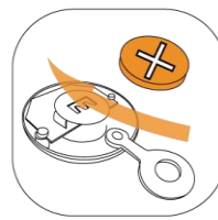
Install new CR2032 battery
